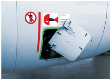
Damage caused by partial loss of Oil Filler Door
