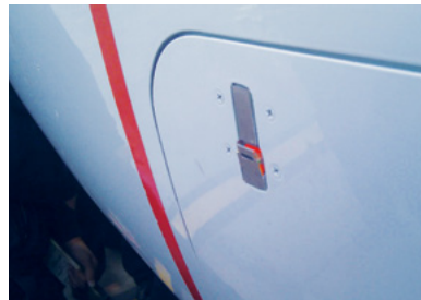
Pre-mod showing Refuel Filler Door not fully closed leading to scooping effect
